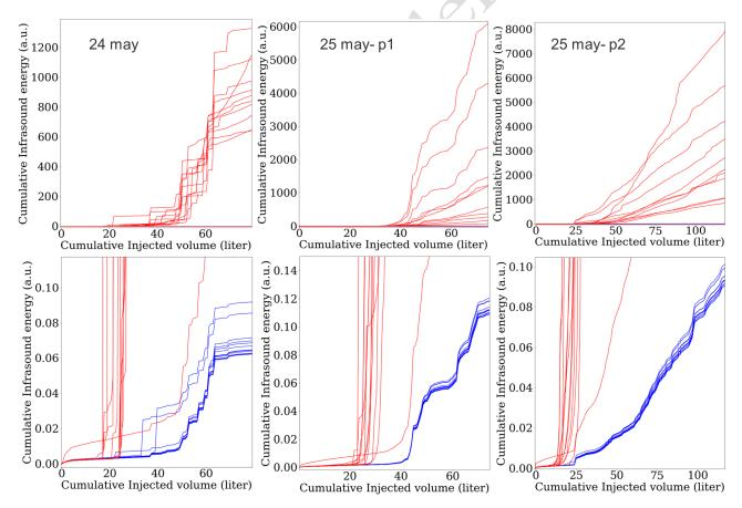
Figure 2: Dependence of fluid injection rate on infrasound energy release. E1-OT is situated 183 perpendicular to the fractured zone and is intersected by it whereas E1-PDB is lies subparallel to 184 the fracture and further away than E1-OT. The infrasound energy measured by E1-OT (red) 185
