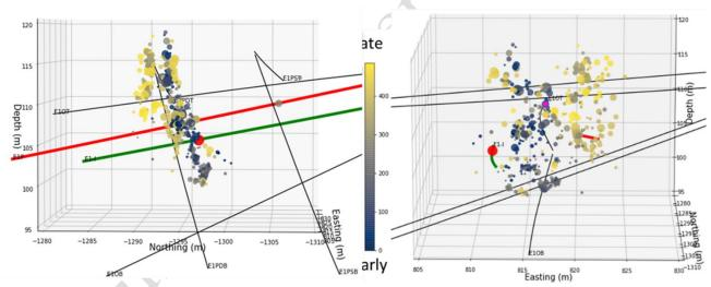
**Figure S7**: Relative orientation of wells E1-OT and E1-PDB microseismic cloud (combined 24 May and 25 May) with the injection and production wells (green and red, respectively).
