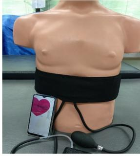
**Figure 1** prototype of respiratory muscle training version II (TU-breathe V. 2)
