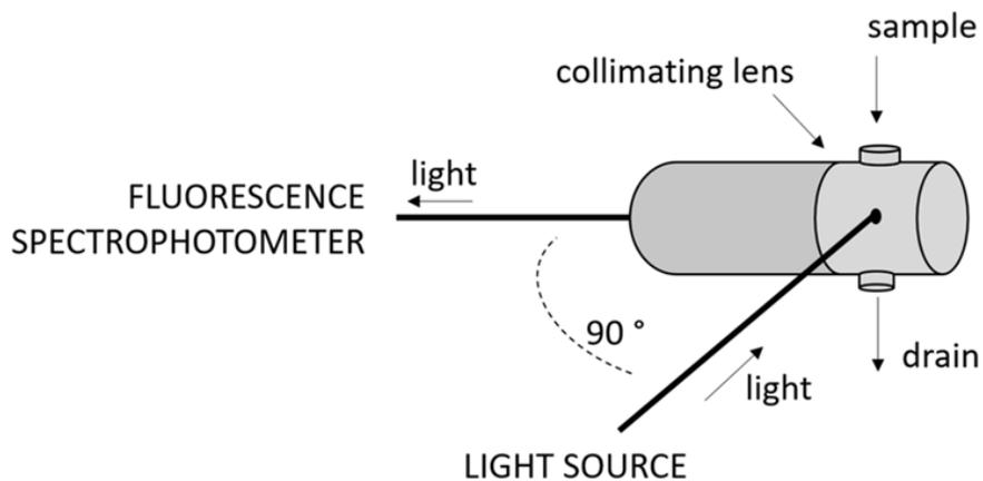
**Figure 2** Experimental setup used with the fluorescence sensor.
