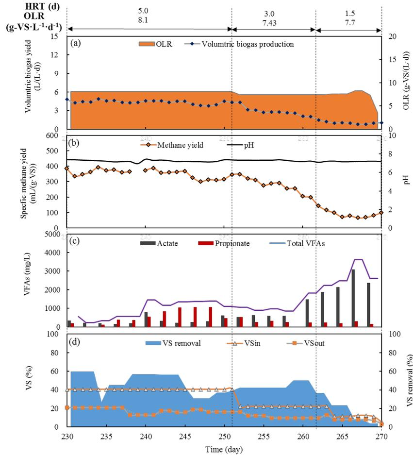
**Fig 3.** CSTR performance under stable and disturbed states targeting HRT: (a) volumetric methane production, (b) methane yield and pH, (c) total VFAs, acetate and propionate and (d) VS in, out and removal
