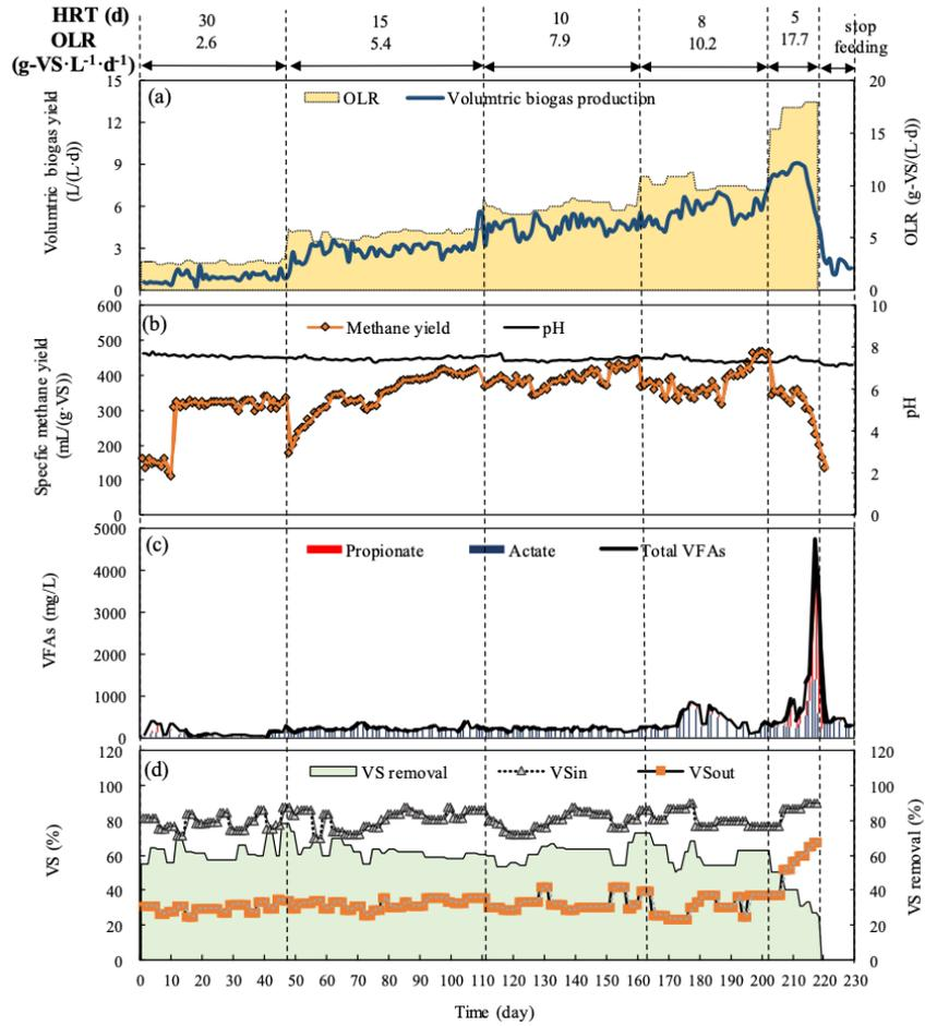
**Fig. 1** CSTR performance in long-term operation under stable and disturbed states targeting OLR: (a) volumetric methane production, (b) methane yield and pH, (c) total VFAs, acetate and propionate and (d) VS in, out and removal
